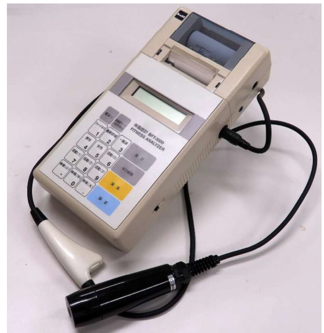
Figure 1. Near Infrared Interactance spectroscopy.
